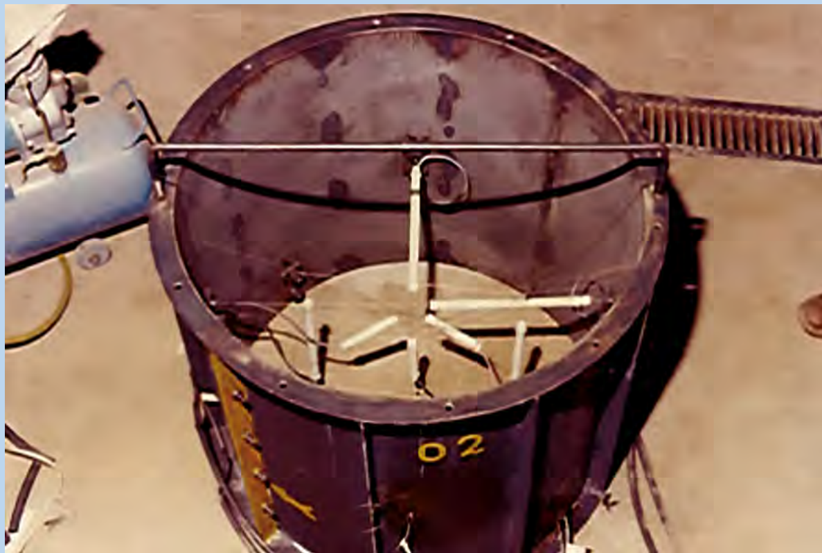
Fixing the strain meters in the mold and casting part of the specimen with a set of stress meters at Itaipu Laboratory (From Andriolo's Archive, 1978)
