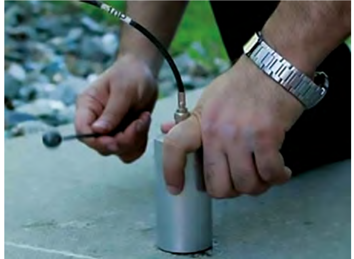
Impact Echo used for concrete inspection [10-03]
