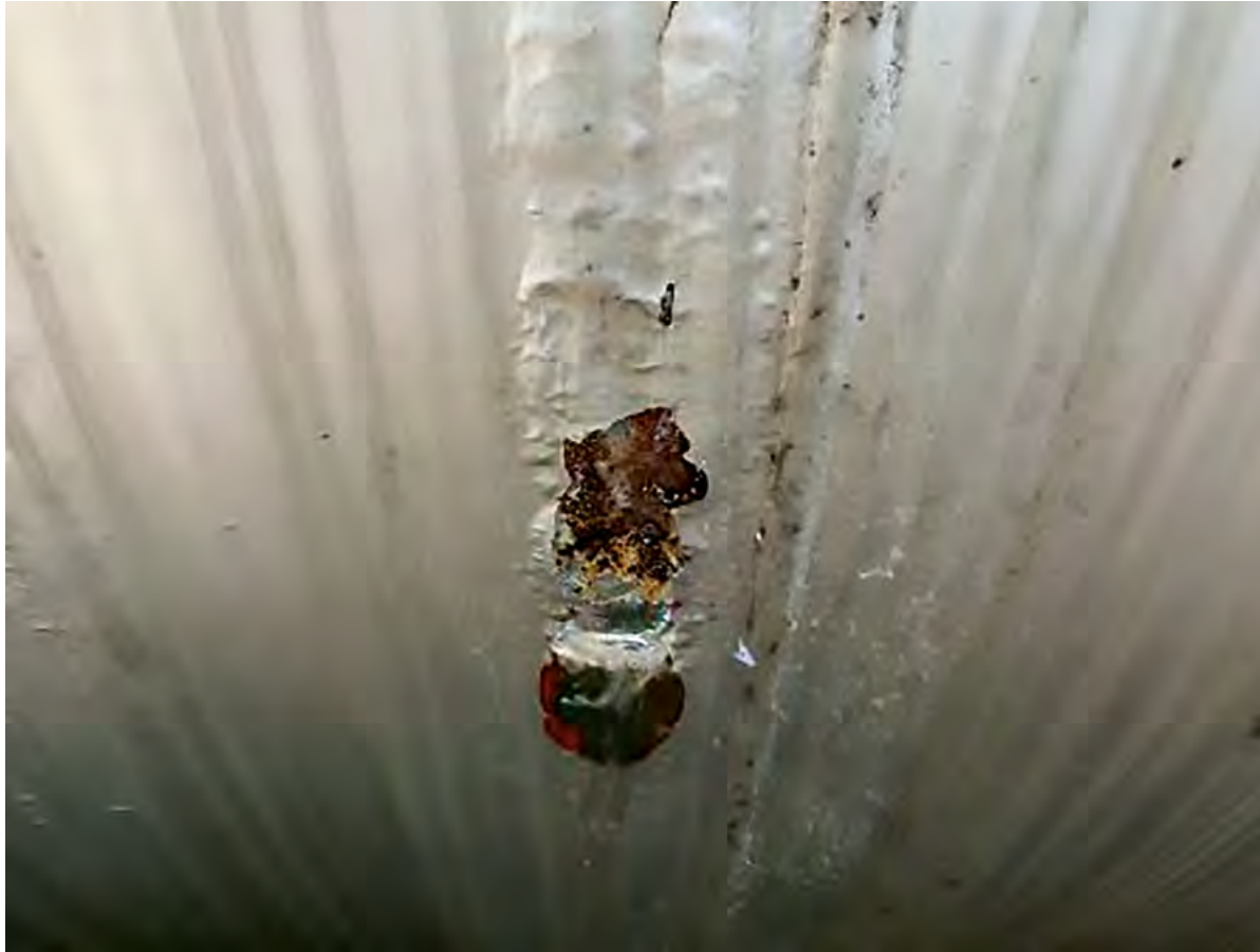
Corroded part of a pipe outer surface (from Ref. [09-02])
