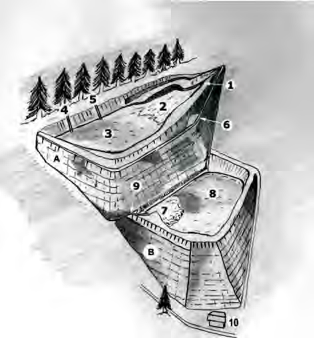
Graphical representation of the Prestavel basins: (A) upper basin; (B) lower basin; (1) cyclone, (2) sandy deposit, (3) silty deposit, (4) drainage service, (5) emergency drainage, (6) service road, (7) sand cone, (8) silty deposit, (9) drainage from the upper basin, (10) caretaker's house.
