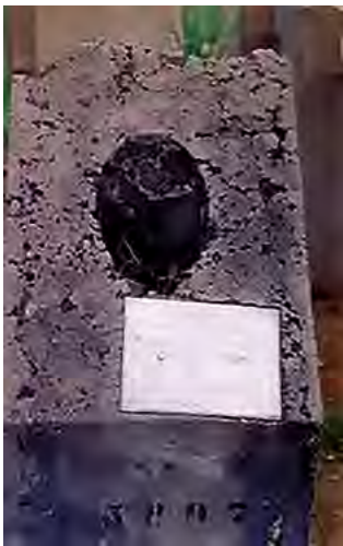
Concrete blocks that were cast (1972 – at CESP Laboratory-Ilha Solteira-SP-Brazil) to check the behavior due to the use of different cement-pozzolanic material and aggregates. The block-specimens were observed in between 1972-2012 (Andriolo’s Archive)
