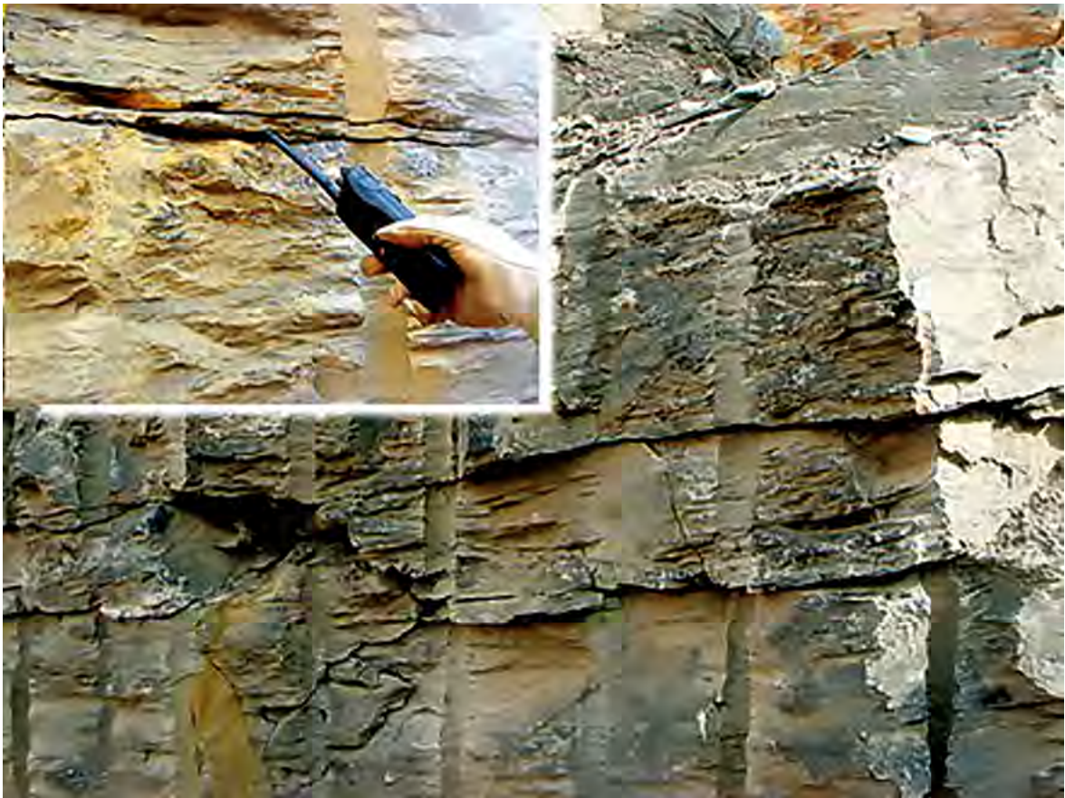
Discontinuities through chlorite schist with chlorite gauge whose influence was only known during excavation
