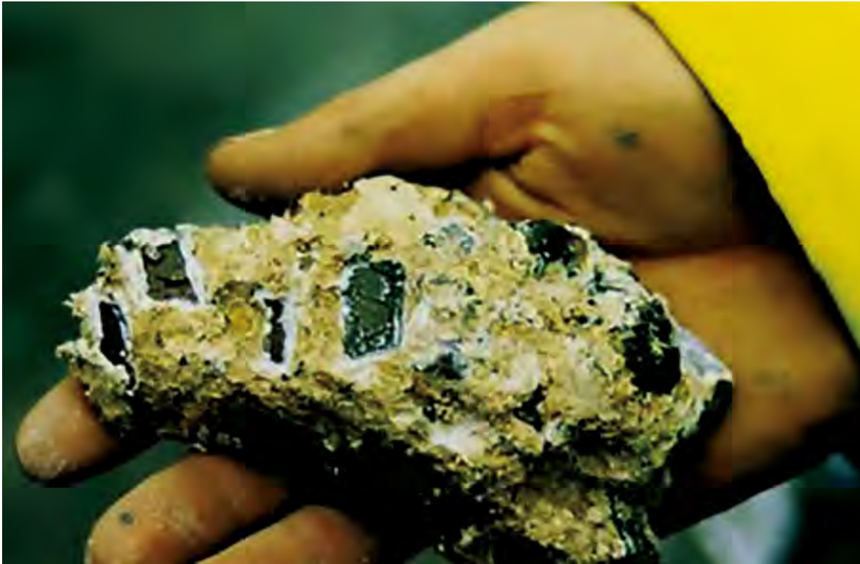
Degradation of concrete caused by sulphate (thaumasite) attack
