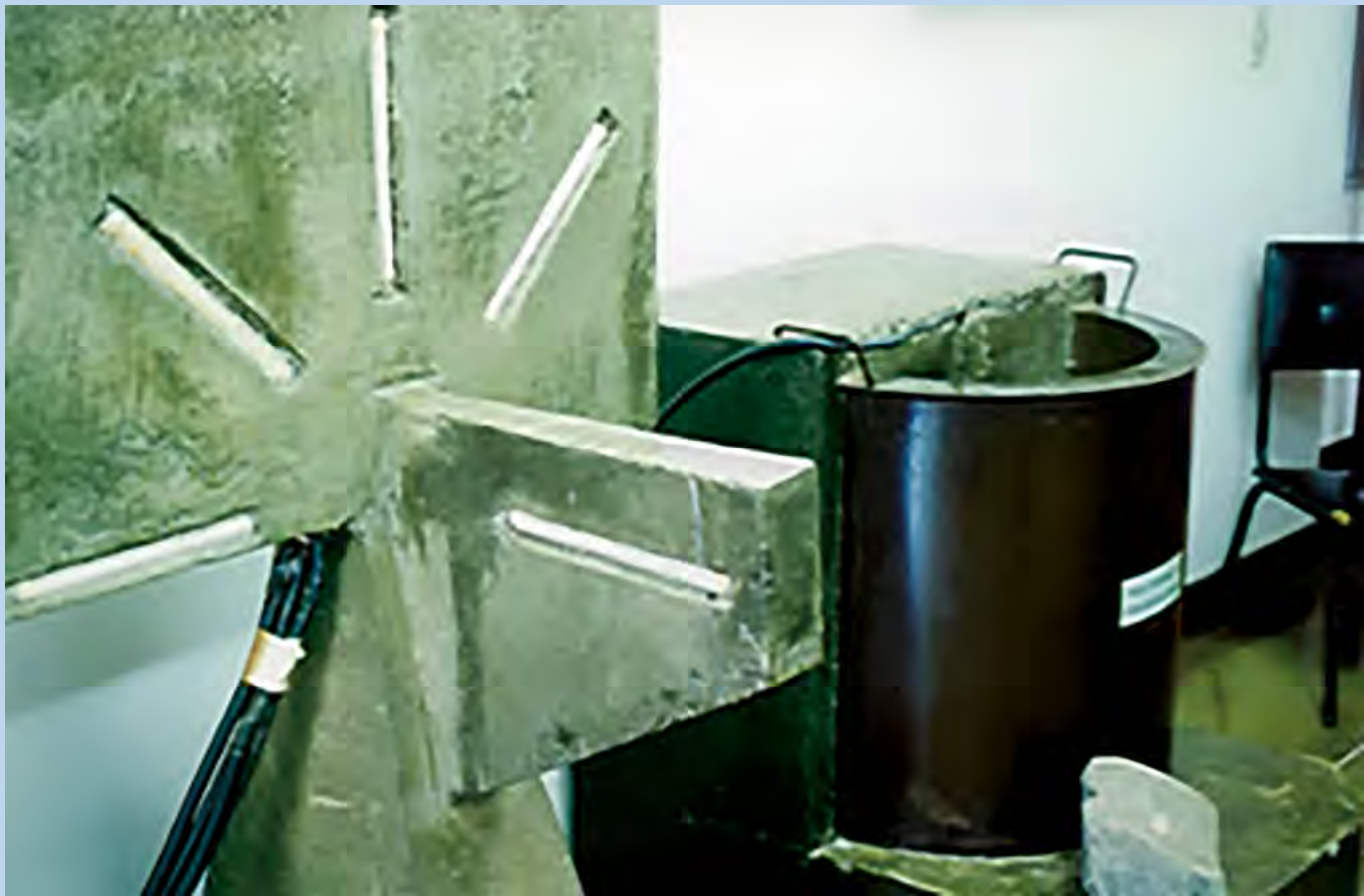
A model with a strain meter spider and autogenous box for training at Itaipu Laboratory (From Andriolo's Archive)
