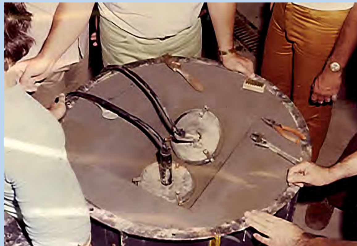
Fixing the strain meters in the mold and casting part of the specimen with a set of stress meters at Itaipu Laboratory (From Andriolo's Archive, 1978)
