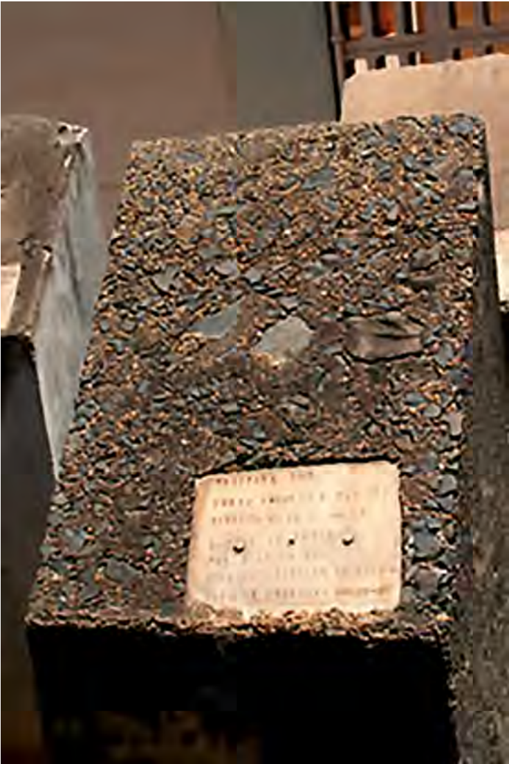
Concrete blocks that were cast (1972 – at CESP Laboratory – Ilha Solteira – SP, Brazil) to check the behavior due to the use of different cement-pozzolanic material and aggregates. Inspection during December, 2021 (Andriolo’s Archive)
