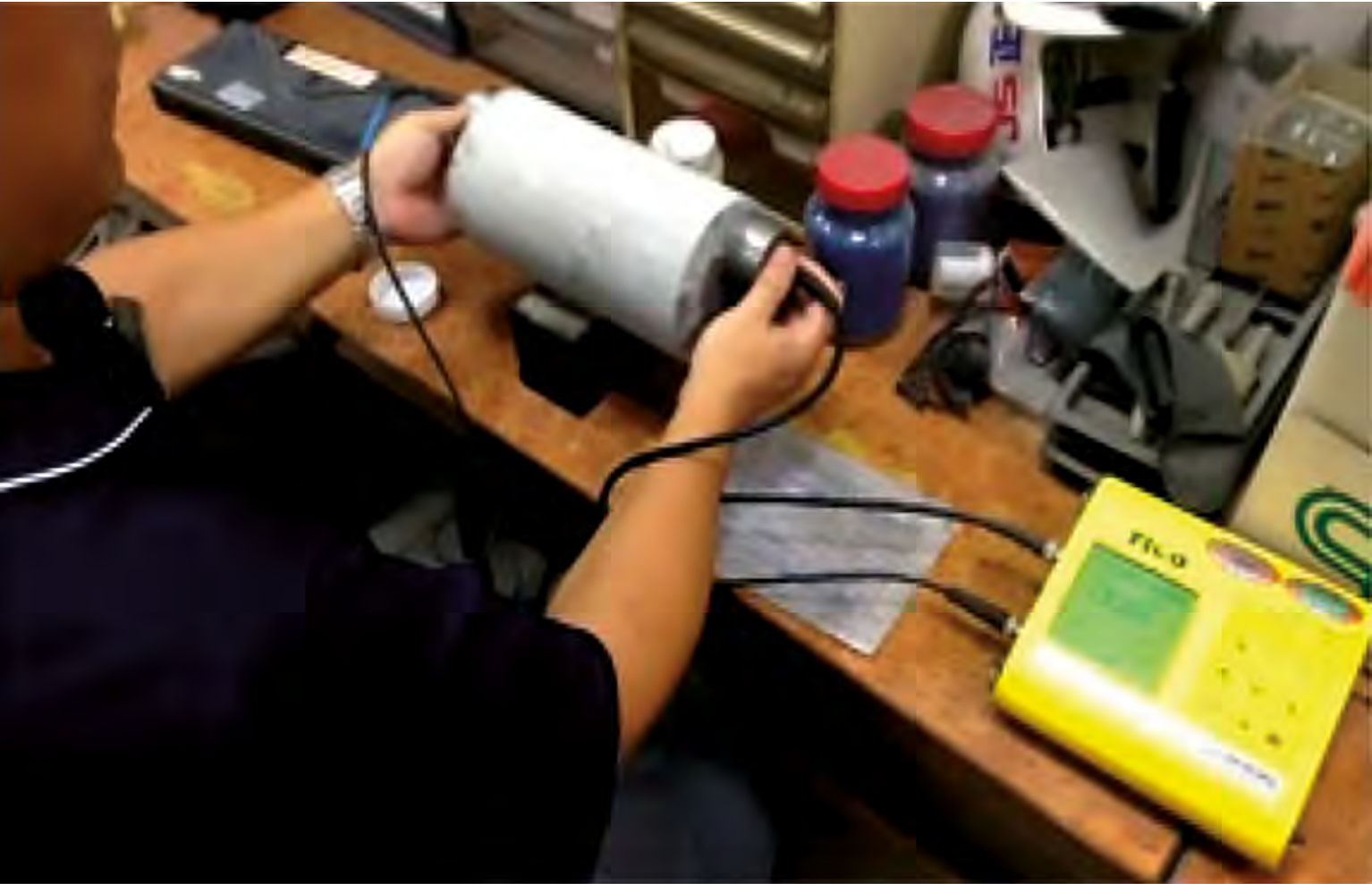
Ultrasonic Pulse Velocity (UPV) method being used for evaluation of concrete properties [10-03]
