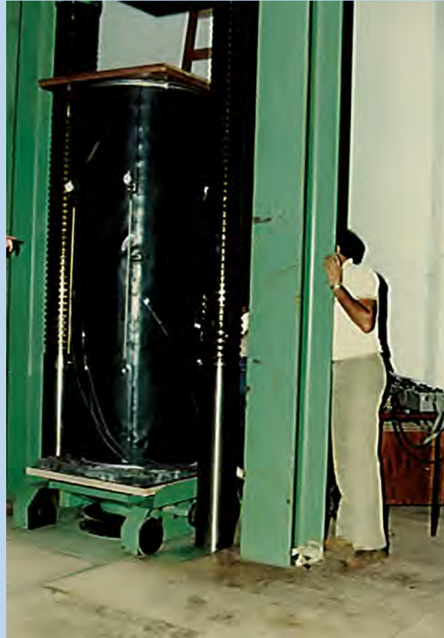
Testing the large specimen with different the transducer meters at Itaipu Laboratory and a view after test (From Andriolo's Archive, 1978)
