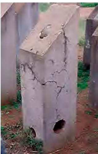
Concrete blocks that were cast (1972 – at CESP Laboratory-Ilha Solteira-SP-Brazil) to check the behavior due to the use of different cement-pozzolanic material and aggregates. The block-specimens were observed in between 1972-2012 (Andriolo’s Archive)
