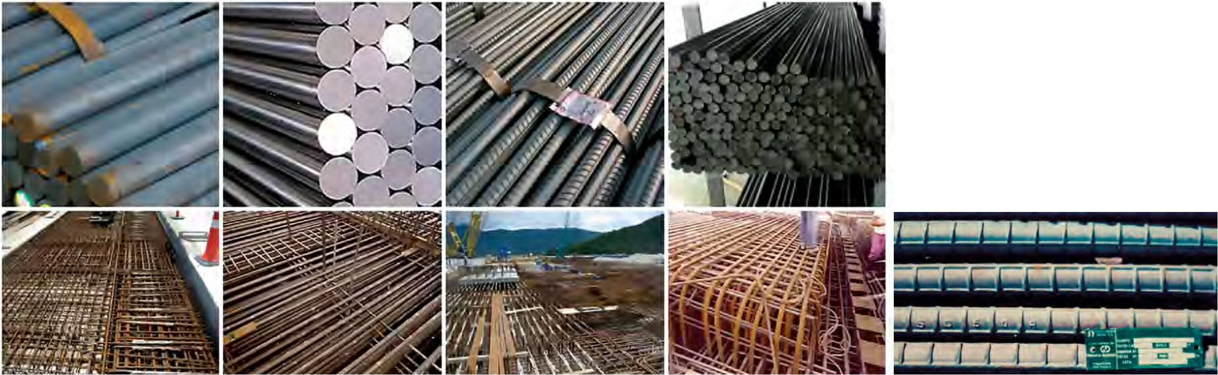
Types and identification of re-bars [03-01 & 03-03]
