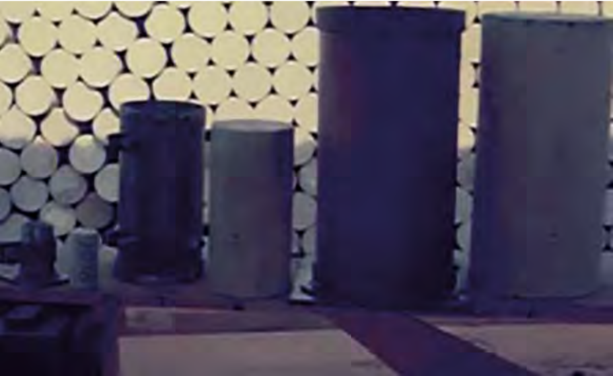
Concrete specimens with different sizes due to the Maximum sizes of the aggregates
