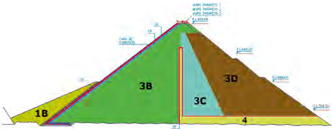
Porce III CFRD Dam Transversal Section in Colombia – H:151m; V:4,155,000 m 3 [04-06]
