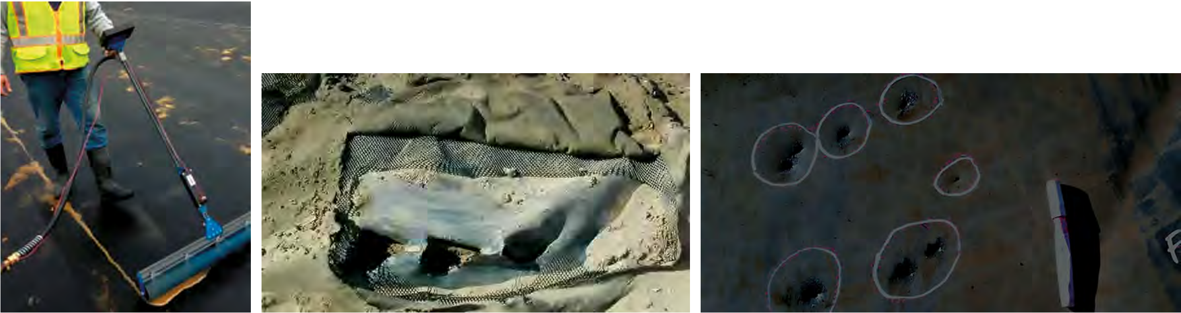
Poor preparation of the subgrade or, in the case of a covered geomembrane, the wrong selection of the type of cover and/or its placement can heavily damage a geomembrane
