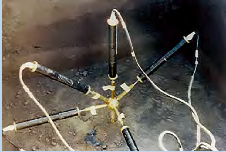
Installation of a strain meter spider and autogenous box in a confined zone at Tucuruí Project (From Andriolo's Archive, 1982)
