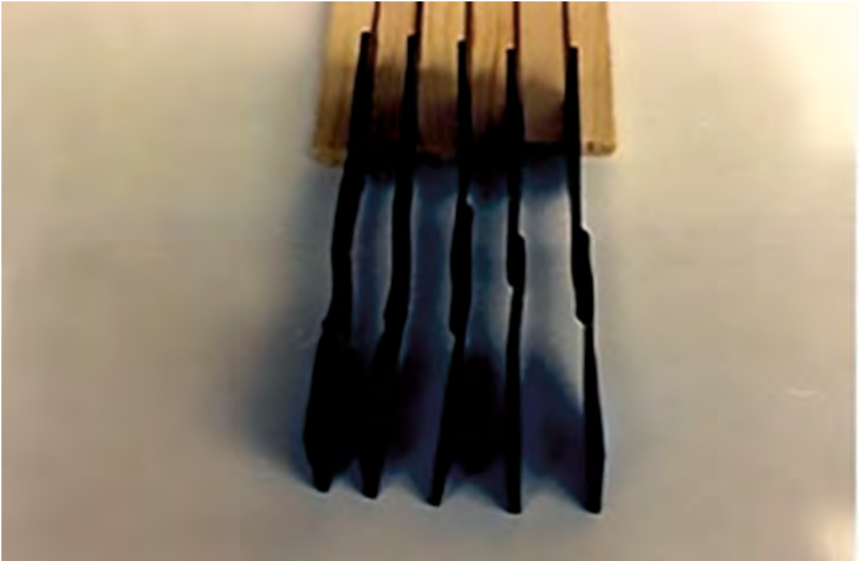
Tensile and tear specimens for tests at Itaipu Laboratory in 1989 on a PVC membrane used in concrete precast panel for the Capanda RCC Dam in Angola (Andriolo's Archive) [03-02]
